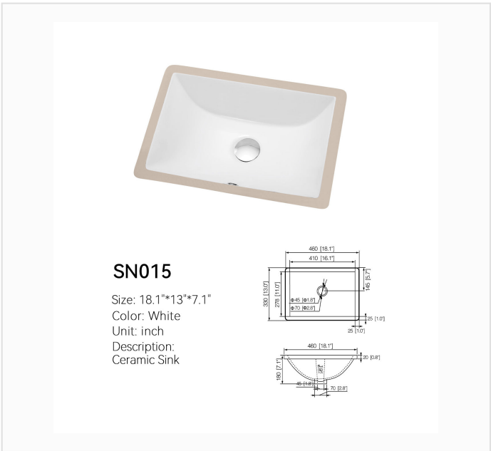
DIMENSION DRAWING · INCH [MM]
