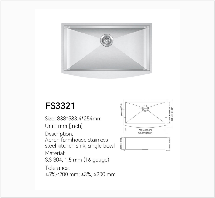
DIMENSION DRAWING · INCH [MM]
